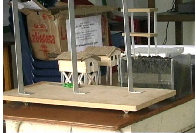
Picture 6. Didactic models with the purpose of showing the vibration of the ground (seismical table), liquefaction (sand boxes) and the housings turn over (miniature model).
