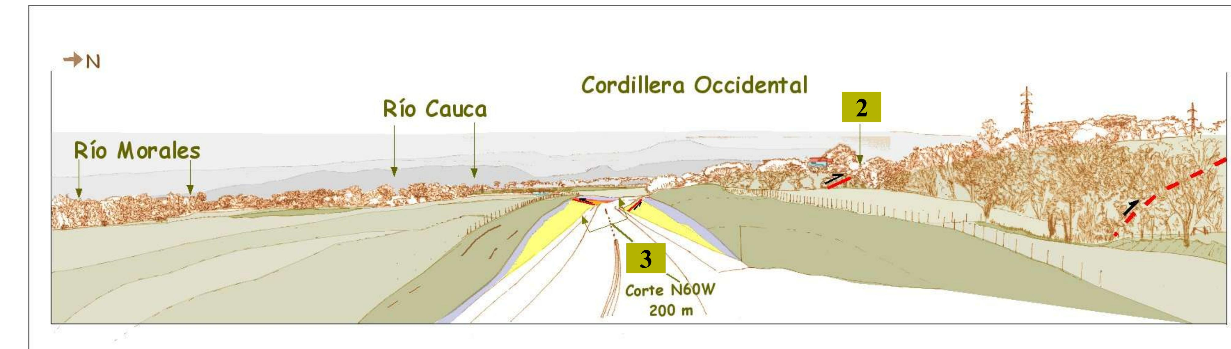
Further events are expected to occur on the west vergent faults (low-angle blind faults), affecting the youngest Cauca river sediments toward the Occidental Cordillera. The east vergent faults are progressively cutting older and deeper geologic units toward the Central Cordillera.
